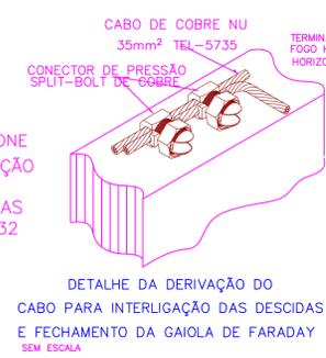
DETALHE DA DERIVACAO DO CABO PARA INTERLIGACAO DAS DESCIDAS E FECHAMENTO DA GAIOLA DE FARADAY SEM ESCALA
